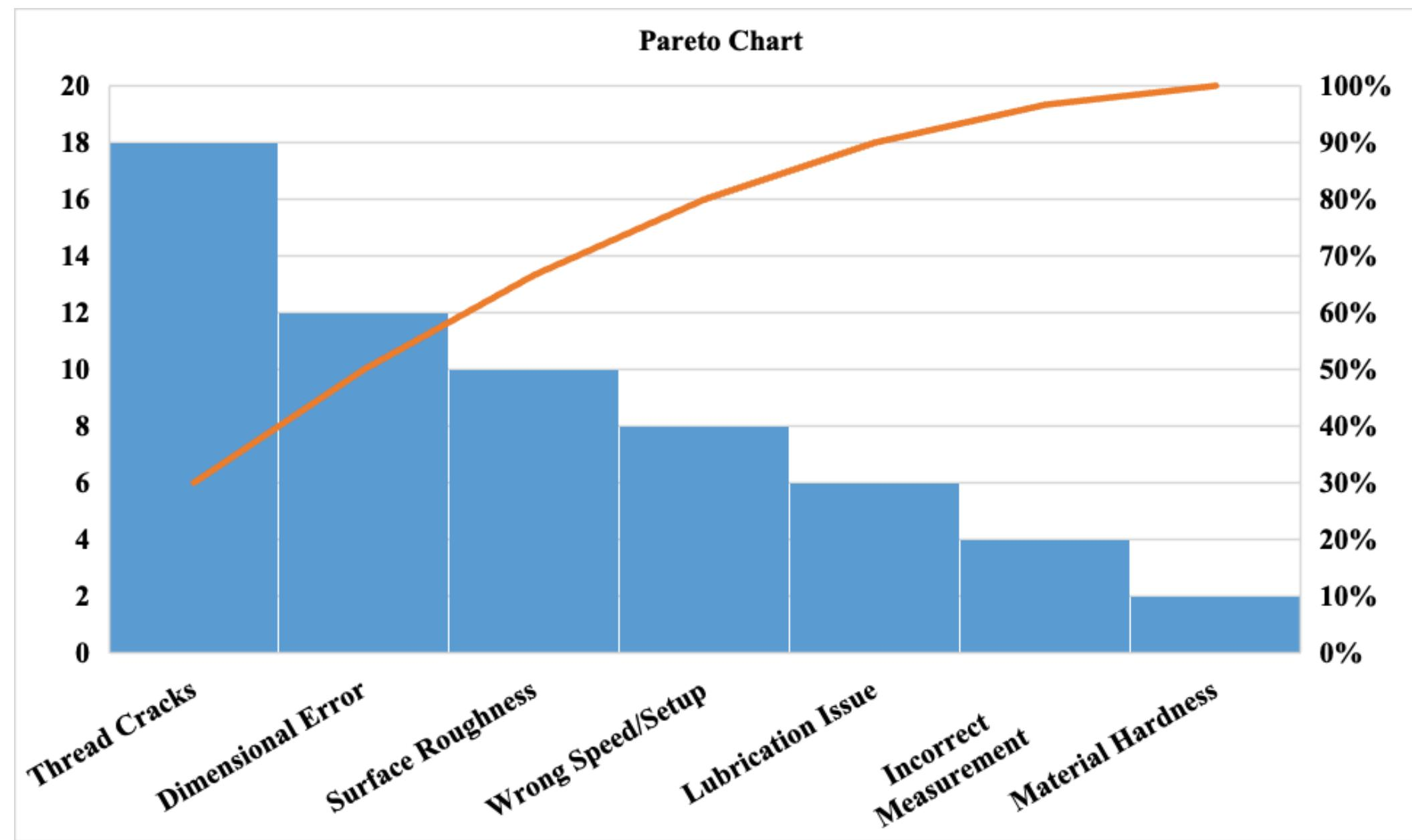
The Pareto Chart shows that Thread Cracks is the most significant defect, accounting for 30% of all reported issues. According to the 80/20 rule principle, focusing efforts on the top three defects, Thread Cracks, Dimensional Error, and Surface Roughness will address approximately 80% of the total problems.
